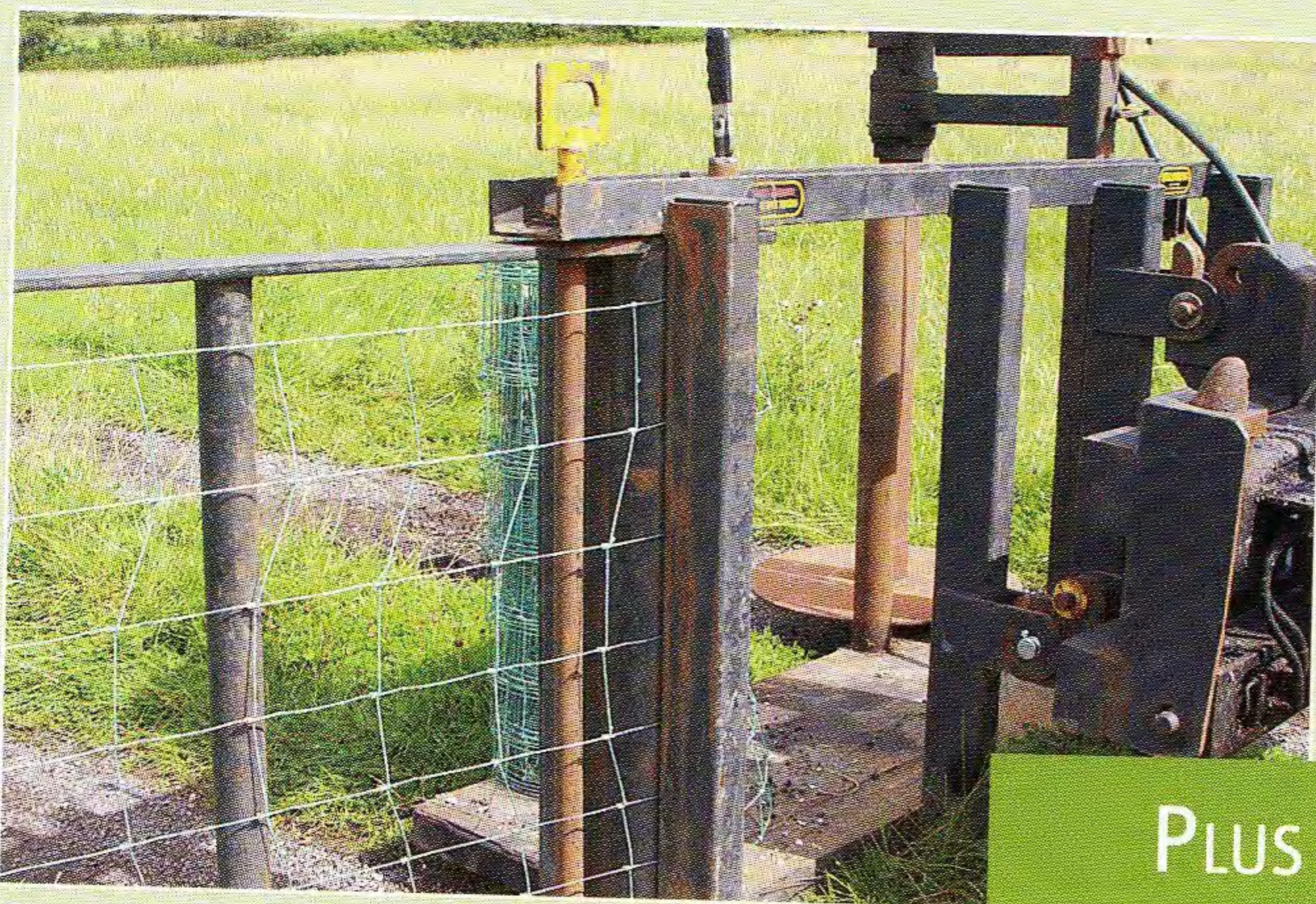
Wire pinch point detail. Note how the hinge grips the wire as the unit is pulled backwards.
